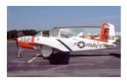
minor changes to meet their unique needs. The most noticeable external difference is the deletion of the small triangular fairing below the rudder. While the Navy was the second T-34 customer, they became its biggest user. They built over 400 of them between 1954 and 1958.
