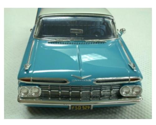
Once I had all the paint stripped off and was happy with the body's clean up, I began to apply white primer to form a base for the Pacific Blue. I put on about four or five coats, then sanded it first with 280, then 320 paper and finally with an old,
