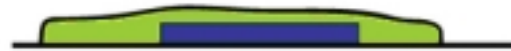
Decal and clear coating finally building up to level at or above decal level.
