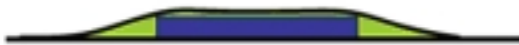
Decal with clear coating starting to build up around the decal and surrounding area.
