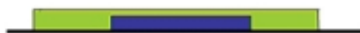
Clear coat above decal level and sanded level with surface (leaving no edge “ridges” at sides of decal.
