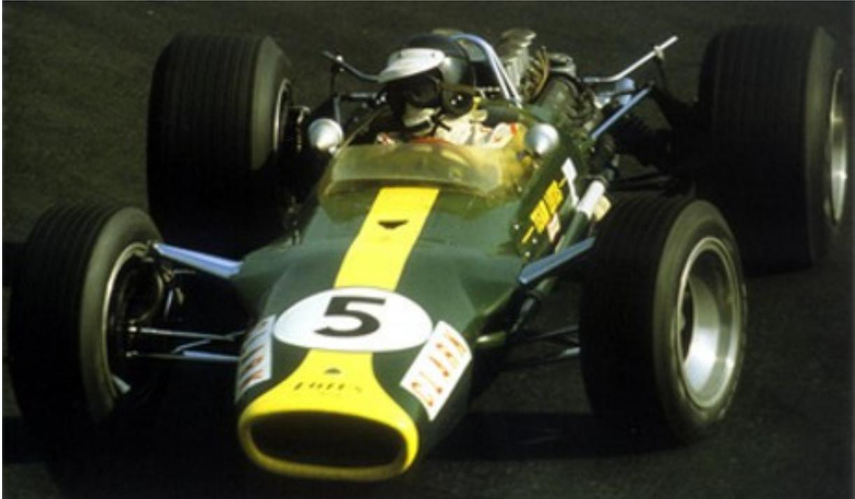
Designed by Colin Chapman, a man whose name in racing history is virtually inseparable from “Lotus”, the 49 has been described as an engine, four wheels, and an austere cockpit all fastened together with absolutely the minimum possible structure. Another description was as a high-speed eggshell. Today the wags often call that era of F1 racing as when “ ...when sex was safe, and driving Formula 1 was dangerous.”
