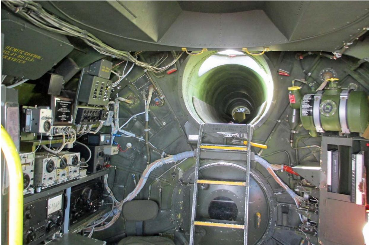
Note the lower hatch, seen in center of the pressure bulkhead. It gives access to the bomb bay, not often used in flight.
