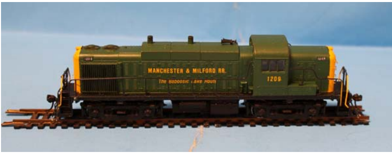
Paul Lessard added horns, MU Cables, grab irons, and cut levers to his 1/87 th Atlas/Big Dawg RS-3M Diesel Locomotive
