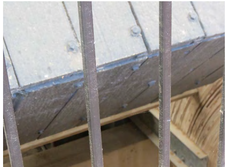
The midship plate extended around the knuckle of the hull and below the waterline for about four feet. They overlapped the ends of the upper casemate plates. It wasn't a particularly neat joint.
