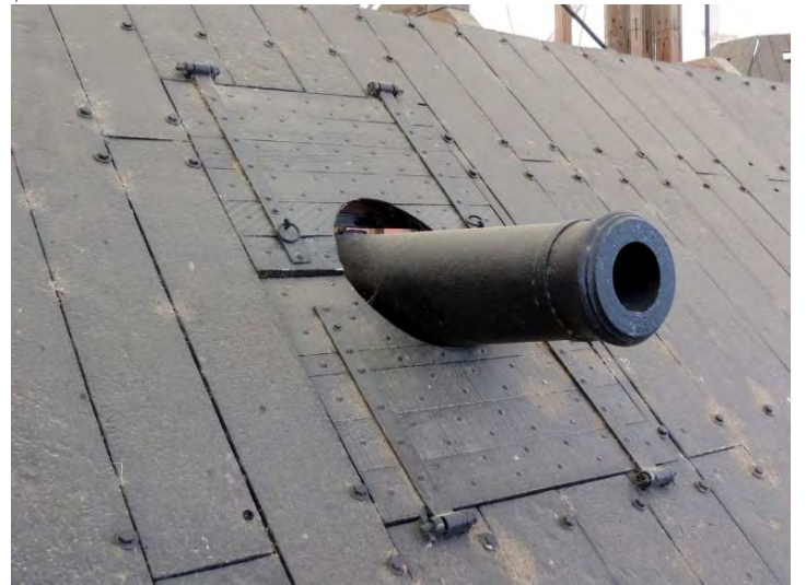
One of the issues I've found with the Flagship kit is how the gun ports are represented. They are raised on the kit but actually flush-mounted on the ship along the plate and the railroad iron sections. Note the pull rings on the upper door but the bottom door simply uses gravity to open it.
