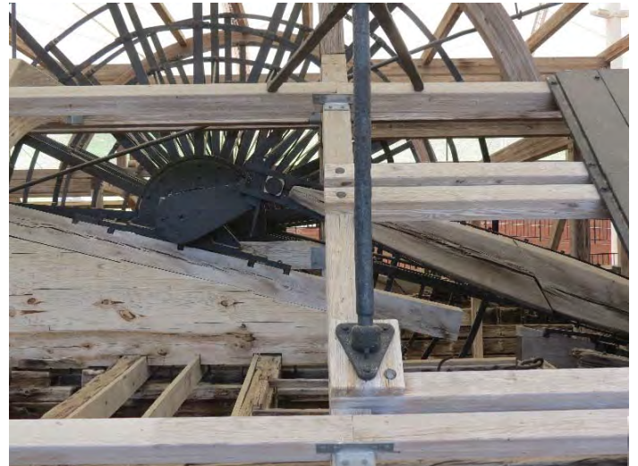
Each engine was connected to a drive shaft connected to the ends of the paddlewheel. I wonder how hard it was to keep the two engines in sync so the drive shafts remained in the same relative position and didn't try to tear the wheel apart. Note in the foreground one of the davits that carried the rowboats. There was one carried on each side.
