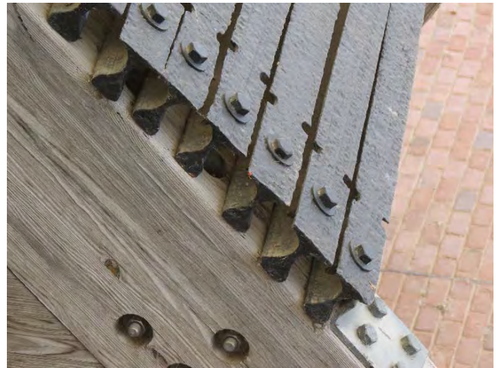
Yet they are much more tightly packed in this picture. Also note that they are mounted with the top of the rail facing inward. It appears that different ironclads did this differently as some had the wider base as the place where the rails were mated to the casemate. A book I am reading on the Arkansas specifically says that the flat of the rails used there were in the inside.
