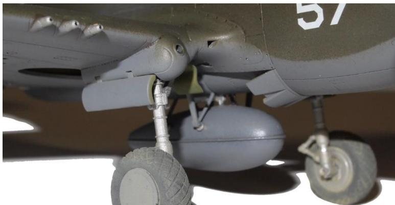
Final assembly gear, gear doors, smoothly. All of these included attaching the, landing and tail wheel, that all went were painted earlier during my painting sessions. I added some plumbing lines to the drop tank and added it with super glue. I now faced adding the clear parts for the lights. I started with the clear parts on the fin. The first one that I cut from the sprue flew into oblivion despite the razor blade being on one side of the
