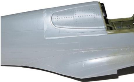
The 0.005" thick plastic was also handy for helping bridge the gaps between the nose plugs and fuselage parts (these parts are plugs on the E-model but vents on the N-model). I wish I had used a 0.005" shim under the forward part of the right nose plug as it took a bit more filler than the left side to become flush. I used another 0.005" shim under
