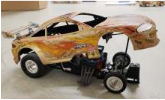
It took George 15 years to finish a 95 Mitsubishi Eclipse funny car. A Charger funny car frame was shortened to accommodate the body. A custom paint job was done using a paint brush that has to be seen up close to be believed.
