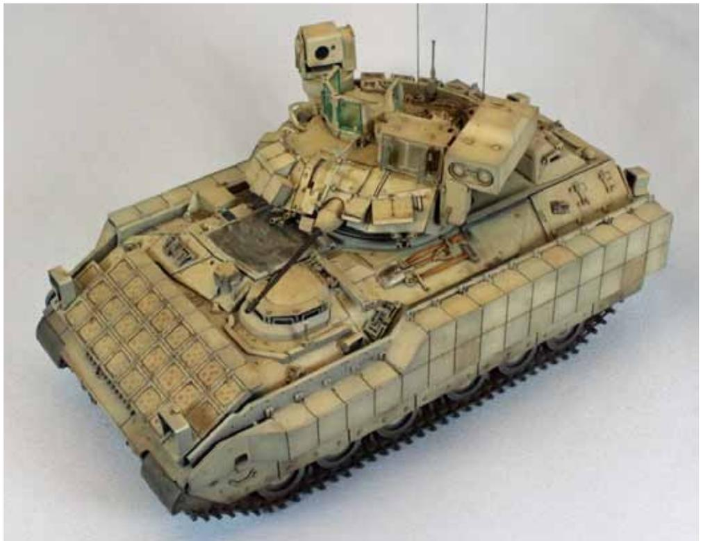
included enhanced identification features, as well as anti-tank missile countermeasures (for first generation wire-guided missiles only) and improved armor protection in the form of ERA.
