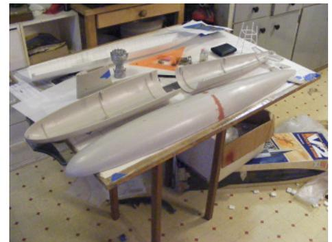
The midships joint of the hull was not hard to deal with, though I'd recommend using a long sanding block to smooth down the area around the joint in order to make sure there is no tell-tale discontinuity in the contours when done. Also, I'd recommend assembling the upper and lower halves as units rather than the instruction's version which would have you build them as fore and aft sections to ensure a more precise midline assembly.
